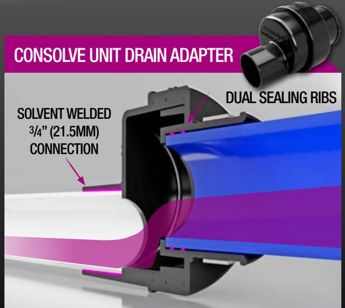
Condensate flows against the critical unglued drain connection which is a common cause of leaks
